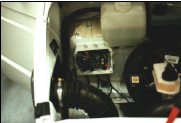
Figure 6 - Interface box in an under-bonnet position
