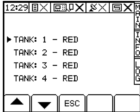
Figure 12 Selecting the "Tank" in the Nozzle Wizard
