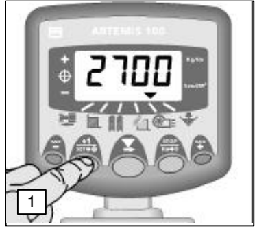
Figure 21: View Fan Alarm Speed
