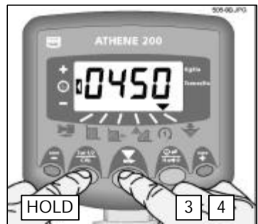
Figure 8b: Set Alarm Quantity
